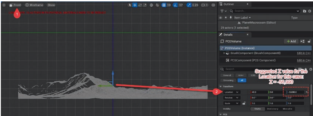
Figure 4-39. Switch to front view, so the PCG volume can be arranged in the center in Z value
